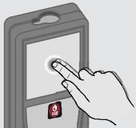
Tap on the display to open an on-screen button or to make a selection. Tapping on the icon in the middle of the bottom line activates the distance measurement or triggers the camera.
