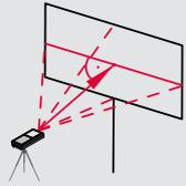
**Aim perpendicular to the horizontal center line of the area. This area must be perfectly flat on the vertical plane.**
