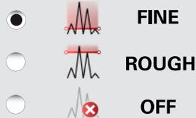
Choose the sensitivity of the levelling, which is needed for some measuring functions. FINE means, that the levelling of the device is sensitive to any small vibrations. Choose ROUGH when working in harsh construction environment with many shocks and vibrations. In this case the accuracy is decreased in correlation with the movements.
